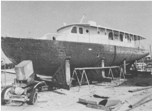
(3) layers Type W14x.437 WIRE PLANK FERRO-MESF1 'R' were used. Note: rub rails were removed.
