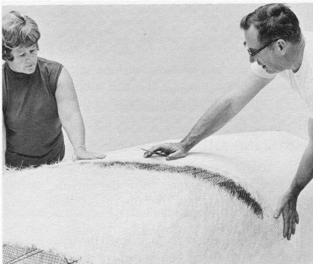
Tailoring fiberglass mat for exterior skin. Note: cotton fabric on right hand side.
