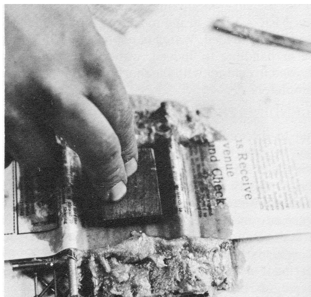
Wood block used to flatten paper and shape fillet over
