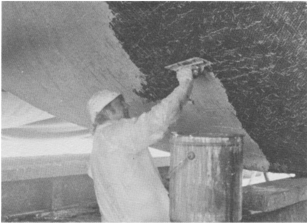
Police all wires for bumps before starting to plaster ... mix FER-A-LITE extra wet to assure penetration.
