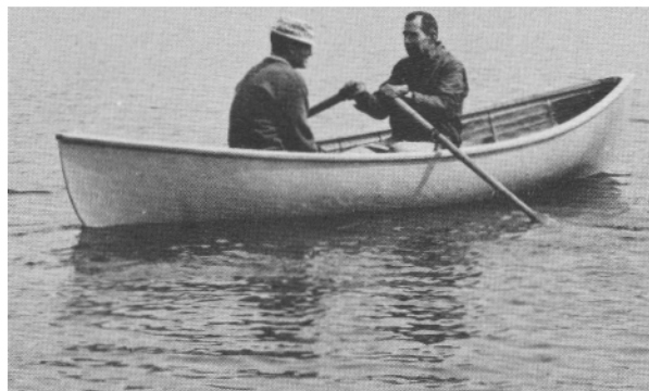
First WIRE PLANK boat built in 1969 was a 13'6" Downeast Peapod which has a 1/8 inch thick Portland cement hull shell.
