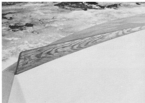
Wood skeg was bonded in place and fastened with large screws.
