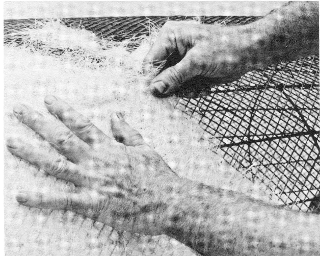
When tearing fiberglass mat grab with a space between fingers.
