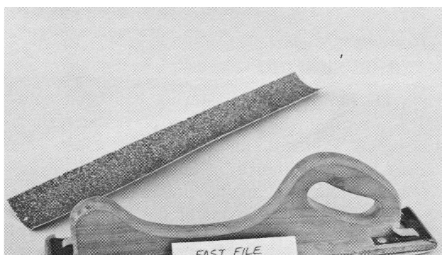
This tool has a quick paper change release feature.
